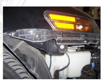
After removing the fasteners on the wheel well, pull down on the skirt and remove the 10mm bolt securing the fender to the body.
