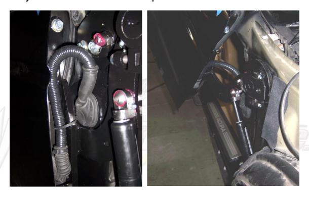
**11)** Cut the inner lip of your fender to make room for the new Vertical Doors hinge. Note: After you have cut the fender use a sander or grinder and make sure the surface is completely flat.
