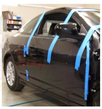
Close the doors and mark the factory location of the door in the horizontal and vertical (pic 1 & 2) positions.
