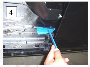
After marking the door and disconnecting the wire harness remove the door factory hinges.
